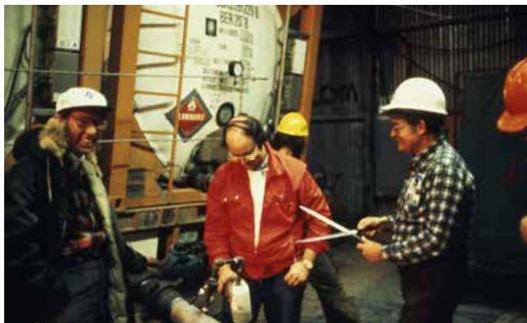
Sampling of gel DRA during first Alaska field test in 1979
